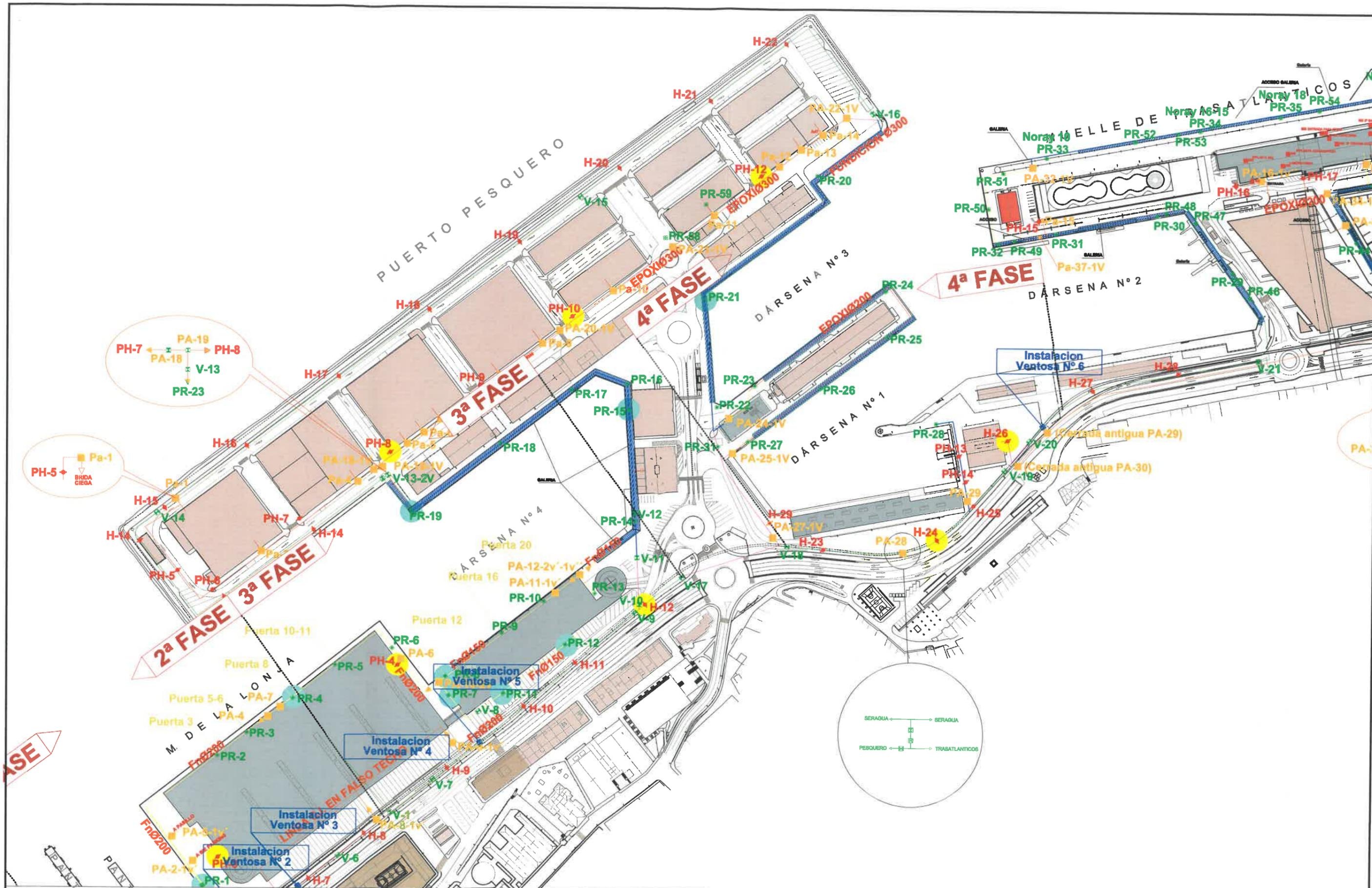
● HIDRANTE SOBRE RASANTE A SUSTITUIR H12, 24, 26, PH3, 4, 8, 10, 12
